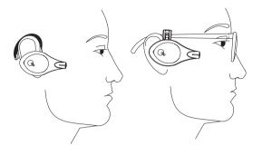
• Insert Loop or Clip from the opposite side of the holding duct if you prefer to wear the headset on the right or left side of your head respectively.
