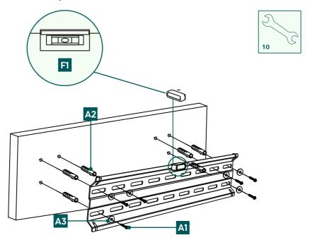
• Attach the wall bracket to the wall as shown above using the enclosed mounting material ([A2] plug, [A3] M8 washer, [A1] 8x60 mm screw and the [F1] spirit level).
