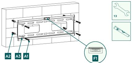
• Attach the wall bracket to the wall as shown above using the enclosed mounting material ([A2] plug, [A3] M8 washer, [A1] 8x60 mm screw and the [F1] spirit level).
