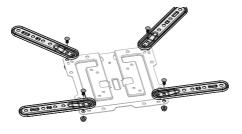
• Mount the adapter plates on the VESA plate using the screws [F1] and nuts [F2] as shown. Use the spanner [G1] for this.
