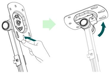
• Turn the ceiling panel from the vertical to the horizontal position as shown above.
