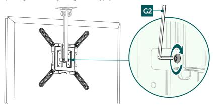
**d)** Secure the TV to the bracket by reattaching and tightening the lower fixing screw that you removed in the installation step **6.1.1 Removing the VESA plate**. Use the Allen key [G2] for this.
